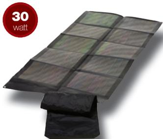
The 30W and 62W solar chargers, built to mil-spec standards, are designed for low maintenance and rugged durability. The SAE plug provides simple attachment to a load. Includes built-in blocking diode to prevent draining batteries. Built-in grommets allow for hanging, mounting or laying in any position. (NOTE: A solar charge controller is recommended with this product!) Accessories not included; each 30W and 62W solar charger comes with a 2-year limited warranty.
