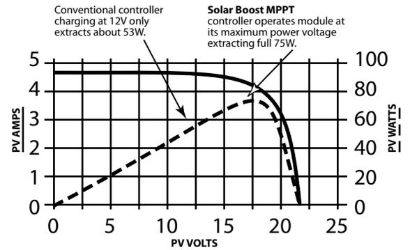
The actual charge current increase you will see varies primarily with module temperature and battery voltage. In comfortable temperatures, current increase typically varies between 10 to 25%, with 30% or more easily achieved with a discharged battery and cooler temperatures. What you can be sure of is that Solar Boost charge controllers will deliver the highest charge current possible for a given set of operating conditions.
